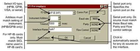
If there seems to be no communication between the HP 14565A application and the dc source, select **Auto Detect** to detect any dc sources connected to your PC. Also, try resetting the I/O interface by clicking the reset button. This also resets the dc source to its default settings.
