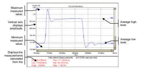
The values in the measurement area at the bottom of the display are calculated from the all of the data that is captured in the display. If horizontal markers have been set, measurements are calculated only from the data between the markers. Refer to Performing Measurements on Waveforms.
